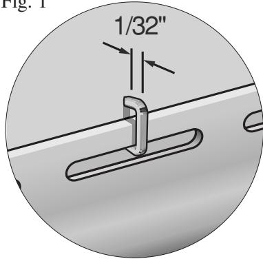
Use aluminum, galvanized steel or other corrosion-resistant nails, staples or screws when installing vinyl siding. Aluminum trim pieces require aluminum or stainless steel fasteners.
