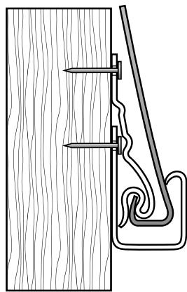
Fig. 1 Starter Strip Inside J-Channel
