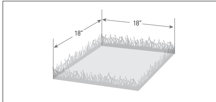
2. Dig or auger a hole with a 10" diameter in the center of this square. Dig or auger it to a depth of at least 24" from the lowest side. Depending on your location, it may be necessary to dig the hole deeper than 24" to get below the frost line.
